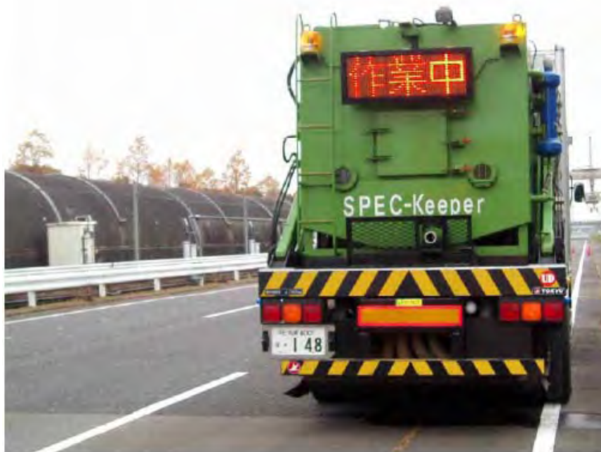
Figure 9. Cleaning machine using high pressure water.
