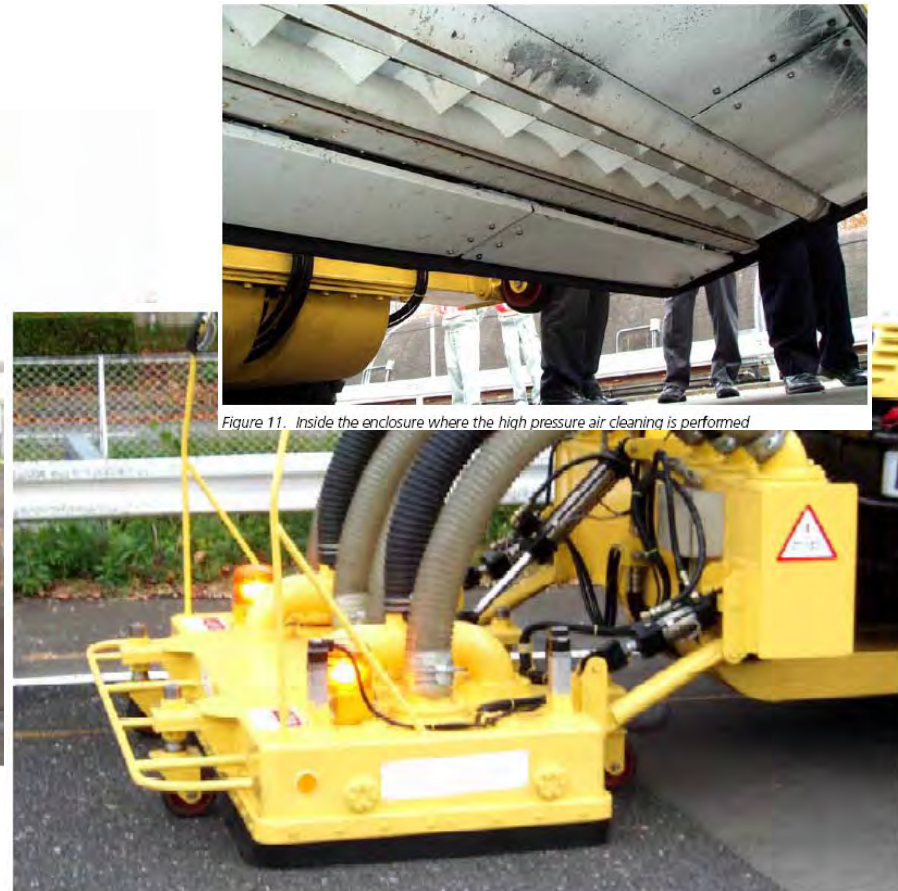
Figure 10. Cleaning machine using high pressure air.
