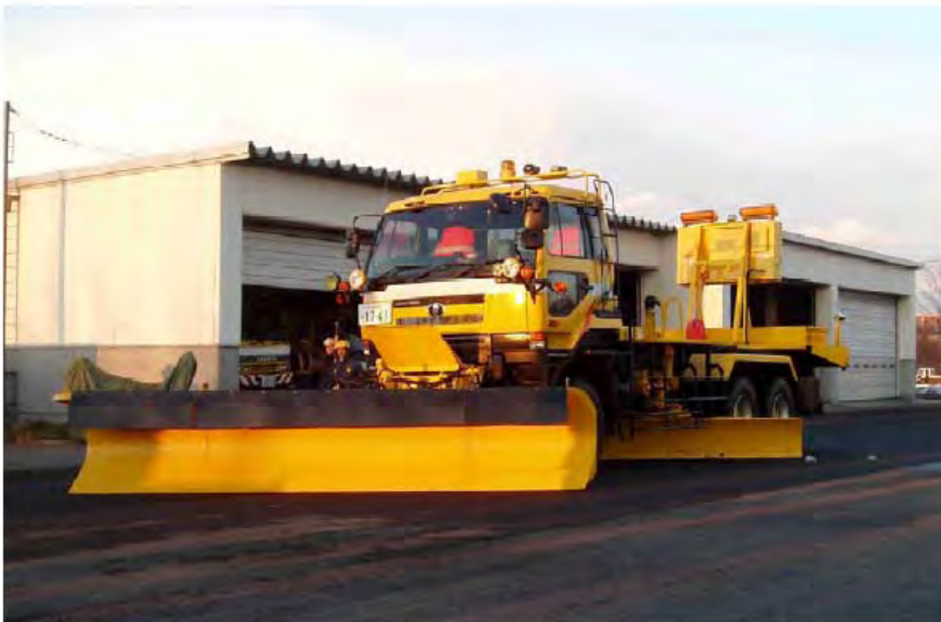
Figure 31. Heavy snow moving material with steel plough used in the Hokkaido road districts.
